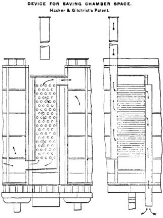
The gases in passing from one chamber to another, are drawn through a leaden tower, called a pipe column. This column is filled with horizontal lead pipes burnt to the sides, and so placed as to continually break the course of the gases, but at the same time allow them to pass.
